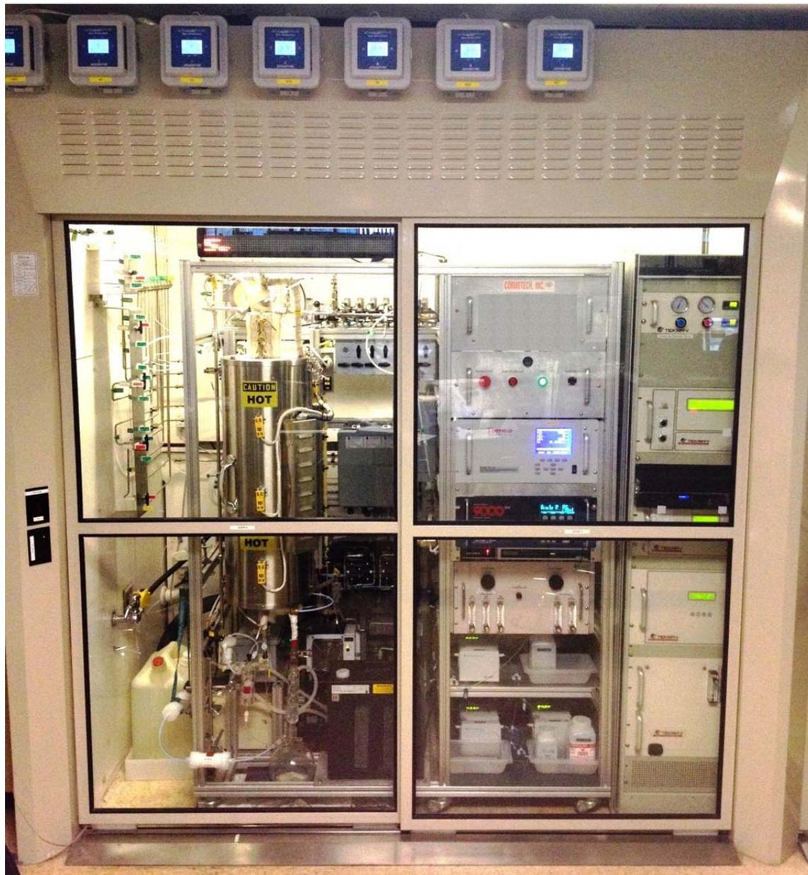
**Figure 2.** Picture of the Cormetech mercury oxidation micro-reactor system. The reactor is enclosed in a floor to ceiling fume hood.
