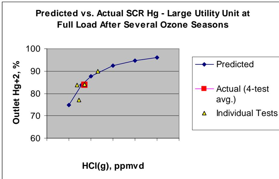
Figure 7 - Full Scale Hg Oxidation Results on Aged SCR Catalyst
