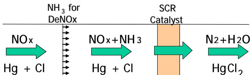
DeNO<sub>x</sub> and Mercury Oxidation Reactions
