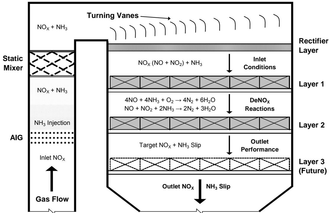
Figure 1. Typical SCR Reactor Arrangement (2+1 Layer)
