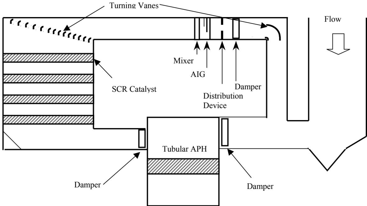
Figure 2: Ammonia Distribution at Catalyst Inlet
