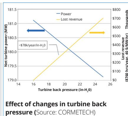
catalytic potential. The graph above shows the effect of reduced back pressure: total MW output increases (blue line) and annual revenue losses decline (yellow line).
