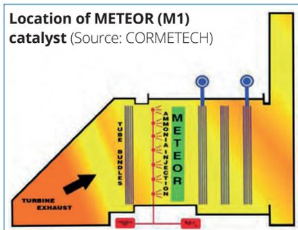
a marked contrast to the traditional approach of separating these functionalities into two catalyst layers.
